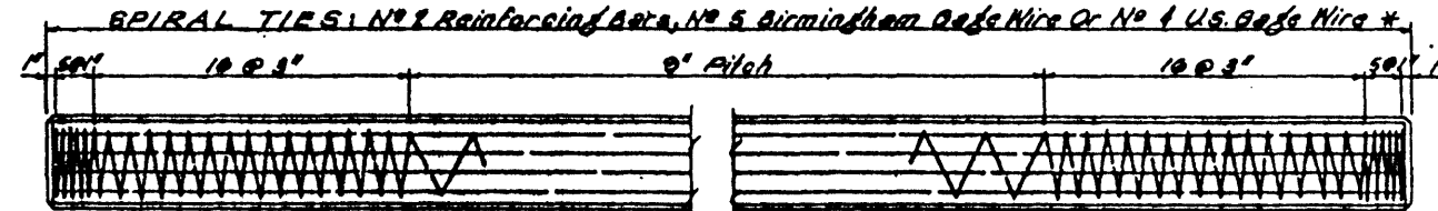
14"x14" PRESTRESSED PILES
