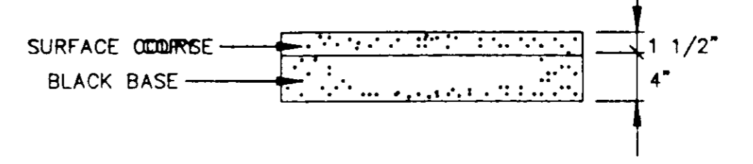
TYPICAL ASPHALT DRIVEWAY REPAIR
