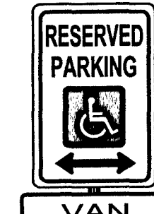
RESERVED PARKING VAN ACCESSIBLE SP-1 (6\"/>
