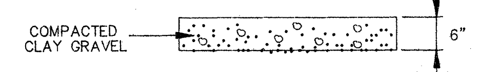
TYPICAL GRAVEL DRIVEWAY REPAIR
