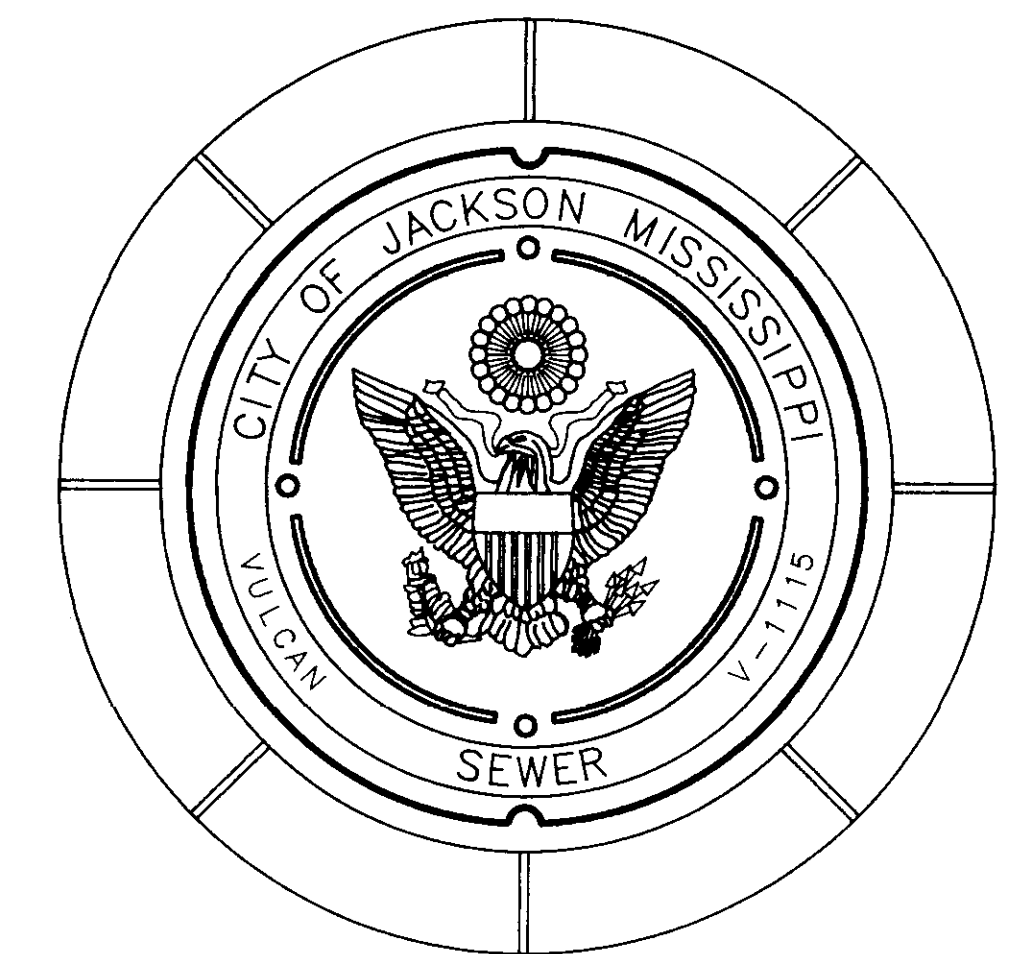
PLAN STANDARD MANHOLE CASTING V-1115 Cover Face
